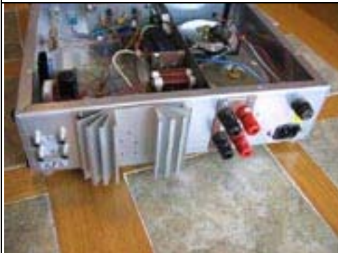
Back end of the unit, showing line input jacks, speaker cable binding posts, and fuse holder. I used a 3A instrument fuse for the 120V input, which is supplied by a removable IEC cord. Note the robust, extruded aluminum heat sink for heat dissipation of the amplifier ICs. Probably a bit of overkill, but it's what I had on hand.
