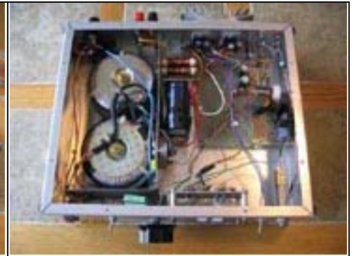
View of the inside. Not terribly elegant inside either. However, the important thing is to keep line-level circuitry well isolated from the power circuitry.
