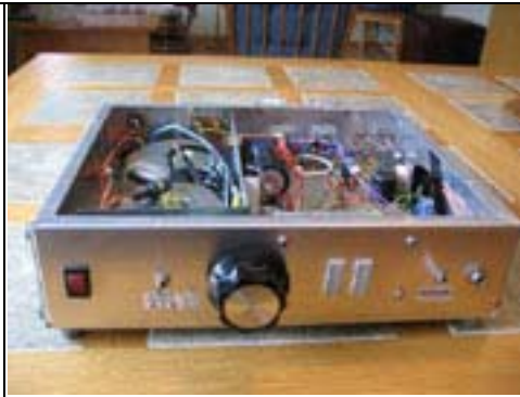
View of the front panel. Controls include main power on/off, volume, two line input selects, speaker/headphone select, LED display VU, and headphone jack. The volume control is a 100k \Omega dual Alps attenuator pot. with detents.
