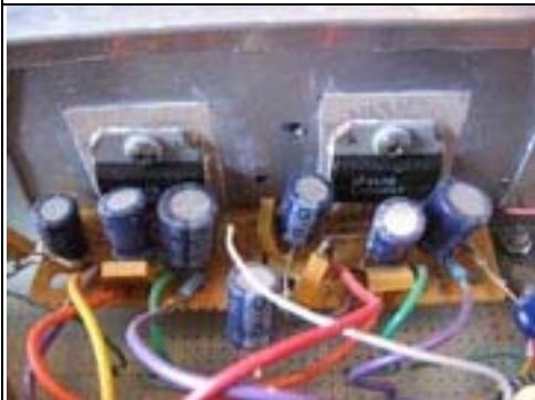
The two LM3886 amplifier ICs bolted to the heat sink, and circuitry. One IC for each audio channel. It's important to keep the components as close to the amp IC as possible, to minimize EMI noise and possible oscillations.
